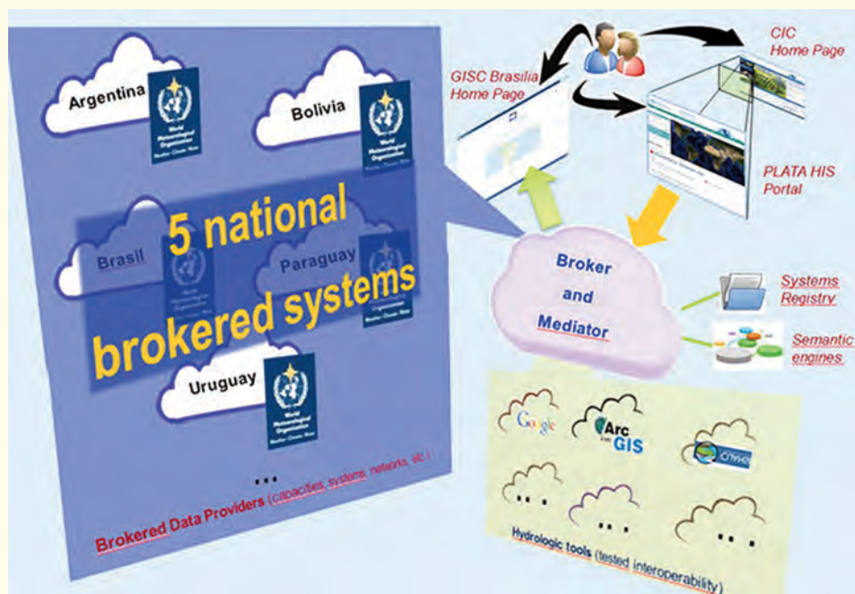
Figure 22 : Discovery and access of hydrological data in La Plata basin
